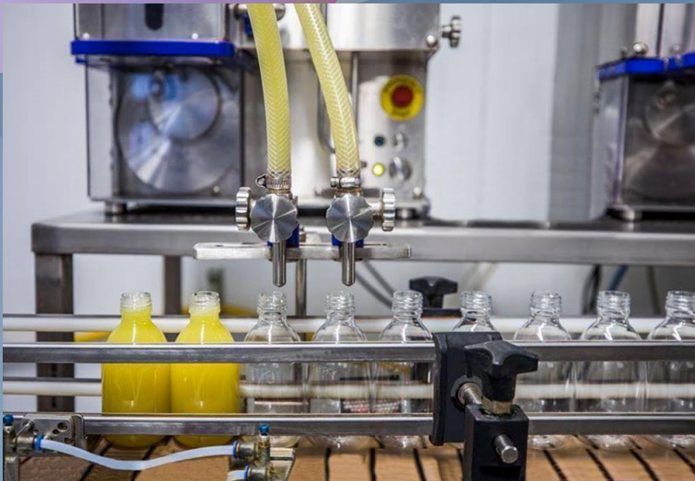
Volumetric Filling machine Model Packmaster II BlueFill line for viscous liquids & creams.
