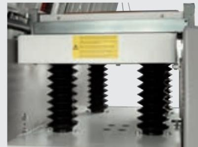
The large dimensioned thicknessing table is mounted over 4 steel screws protected from the dust. This system is extremely precise and ensures stability even when working long and heavy workpieces.
