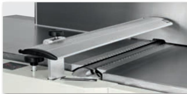
The cutterhead protection ensures the highest safety during working. The protection is foldable.
