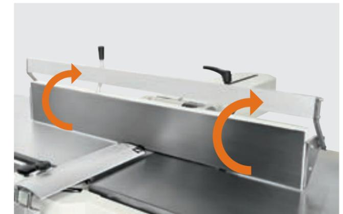
The additional overturning fence, available on request, is recommended to safely machine small workpieces.
