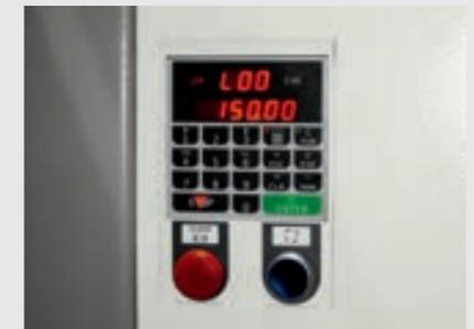
The thicknesser table electronic positioner, available on request, enables fast and precise worktable positionings. With calculator included.
