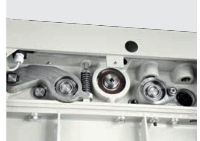
Feed rollers mounted on independent floating ball-bearing bushes.
