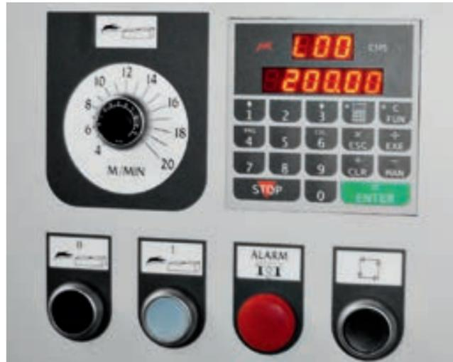
The thickener table electronic positioner, available on request, enables fast and precise worktable positionings.
