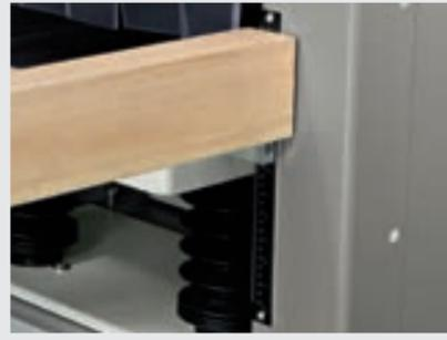
Workpiece measuring device.
