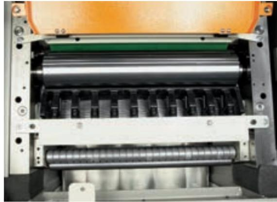
Planer unit with infeed anti kick-back fingers and segmented chipbreakers, serrated steel infeed roller with spiral teeth and rubber coated outfeed roller. Feed rollers are interchangeable. Reduced noise level.
