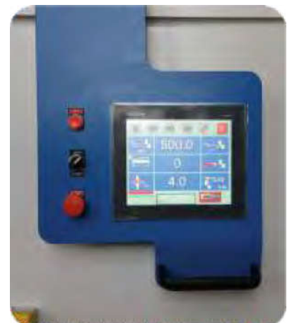
Colour Touch Screen 10.4", movable along machine's length (optional)
