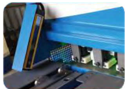
Finger protection with light guards (optional)
