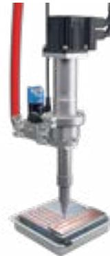
Potting with 2-component trickle resin, e.g. polyester – rotor potting
