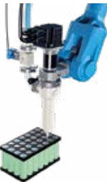
Potting with thermal conductive adhesive, e.g. polyurethane – control element potting
