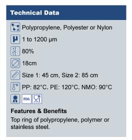
The filter bags distinguish themselves by high flow capability and dirt holding capacity. They come in a broad selection of filtration degrees from 1 to 200 micron in polypropylene and the high temperature polyester bags. We also carry Nylon bags for rough filtrations up to 1200 microns. Less than 30% particles can pass through a bag filter of the same filtration degree.
