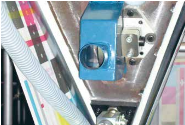
Suction casing mounted on slitter knife in printing press
