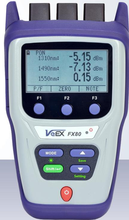
The FX80 family of optical test sets are a new generation of lightweight, handheld and rugged devices for installing and maintaining point-to-point or point-to-multipoint fiber networks. A large, high contrast backlit LCD display simplifies setup and viewing of results in any work environment.
