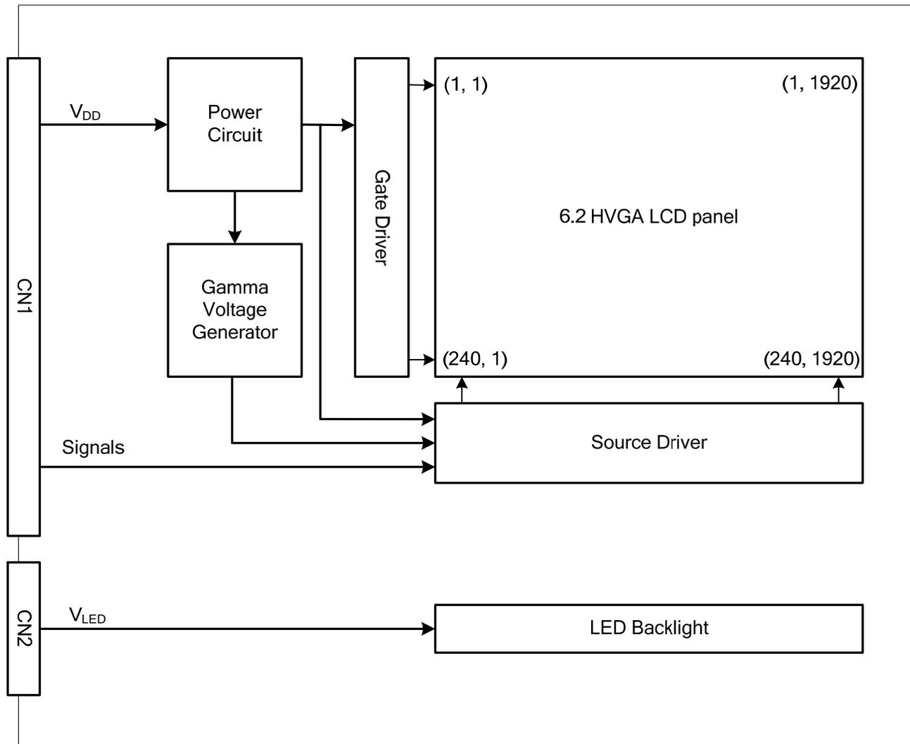
Note 1: Signals are DCLK, DE, and RGB data bus.
