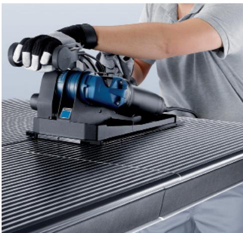
Right-angle cuts using a 90° adjustable blade.
