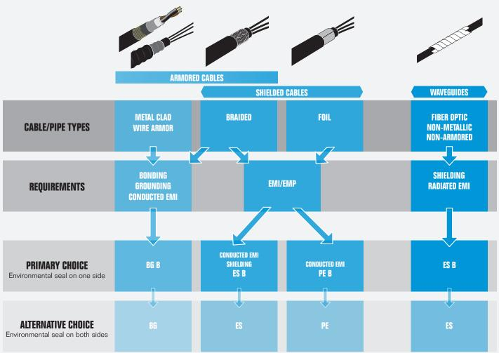
Pipes can use any module type depending on protection required
