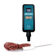
Place the insertion sensor in the food and press the button on the unit. The temperature is now measured and logged every 15 min. After 3 hours or when the temperature drops below 8°C the measuring process is interrupted, and a message is sent. A report of the process is generated automatically and saved on the cloud server.
