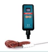
Buffet, preparation of food, dishwasher rinse water etc. The potential of temperature monitoring every 1 min. with display for immediate access to the temperature before logging the data to the cloud server.
