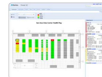
Data Center Health Map A real-time interactive data center health map warns of issues such as hot spot formation, SLA violations, over charges, and loss of redundancy.
