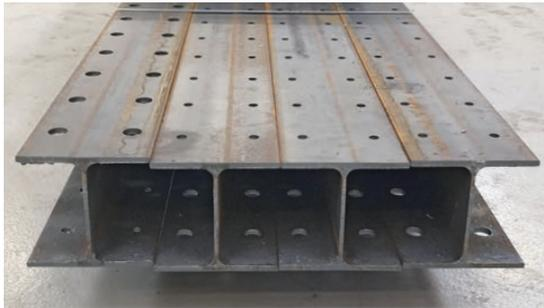
Four days' work reduced to just three hours when we cut HEA 240 beams on our big 3D fibre laser tube cutter. It can cut up workpieces up to Ø355 in aluminium, steel, copper or brass and can handle up to 135 kg per metre. Specifically, this optimises and greatly reduces costs in the customer's own production process, without compromising on quality.
