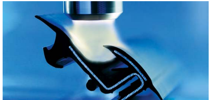
Gap-filling pretreatment of EPDM profiles
