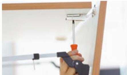
Fronts can be adjusted in 3 dimensions to ensure a pleasing gap design.
