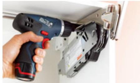
The lift force can be adjusted (according to the frontal weight) using a power screw driver (Pozidriv®, size 2, length 39 mm). To make adjustment easier all AVENTOS mechanisms include a calibrated scale.
