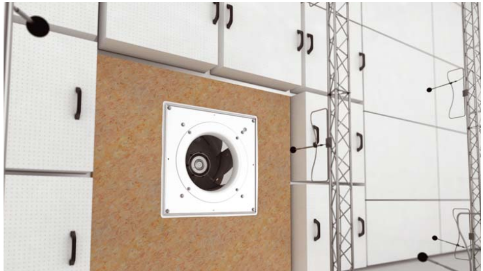
Fig. 1a: Centrifugal fan set up on test stand with free inlet, noise measurement microphones on suction side
