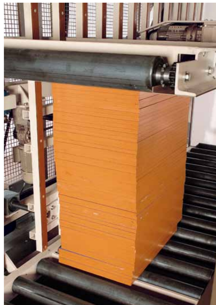
Compattamento pila Stack compacting
