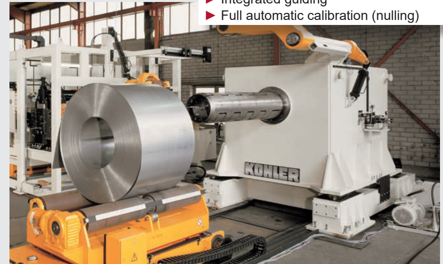
Longitudinal slitting line (Source: Kohler Maschinenbau)
