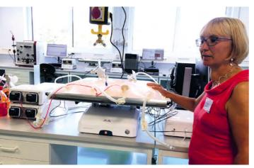
Lotta Ljungqvist is showing the ReadyToProcess Wave 25 Rocker which is a bioreactor up to 25 liters for growing cells.
