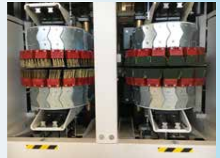
Mix abrasive belt and scotch brite brushes + steel wire brushes Schleifband-Mix und scotch brite Bürsten + Stahldraht Bürsten
