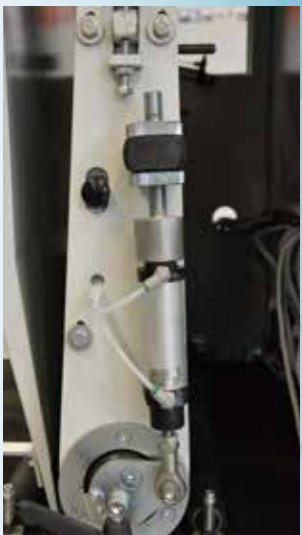
Pneumatic system for belt tensioning Pneumatisches Gurtspannsystem
