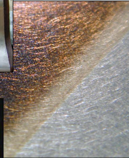
Composite Mold Material after 100 treatments without dirt layer (worst case test)
