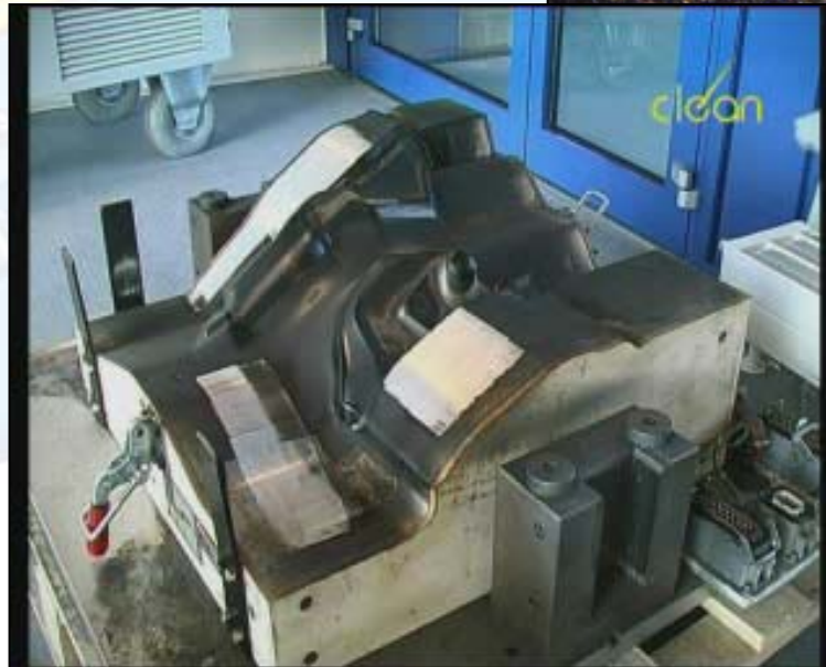
Composite Mold Material after 100 treatments without dirt layer (worst case test)
