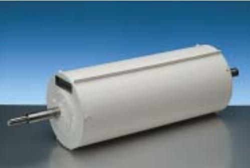
The drum magnet, also called separation drum, contains two sectors: a magnetic and a non-magnetic sector. Around this system a drum rotates onto which the materials are dropped or passed on. For an effective removal, this drum is provided with idlers. The waste is fed onto the magnetic sector of the drum. The magnetic field forces the iron particles to remain longer on the drum. As they leave the drum further down, they can be collected separately.
