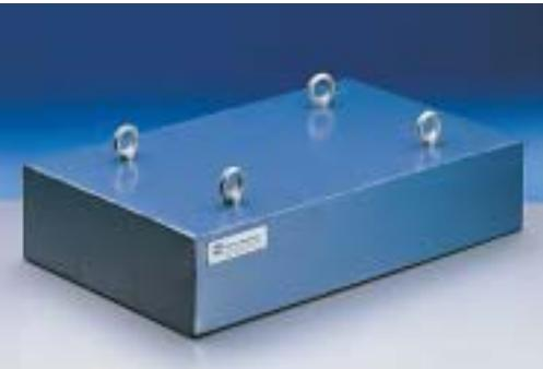
Block magnets can be applied to de-iron material flows on conveyor belts, at a free fall, at vertical or inclined conveyor chutes, above guide plates, etc.
