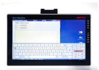
The strong 4 mm anti-glare bulletproof glass layer above the screen withstands acid, cleaning fluids and disinfectants as well as extreme operational demands. Behind the glass there is a projective and capacitive touch panel. A special sensitivity control allows for reliable gesture control – and this even when wearing gloves.
