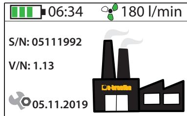
A new serial number is assigned to each blower. You can therefore identify your personal blower by its serial number. The serial number is displayed in the line marked S/N.
