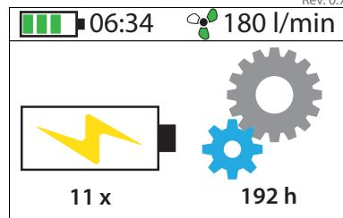
The battery automatically counts every complete charge in the charging station. The respective charging cycles of the connected battery are displayed in the operating information menu.
