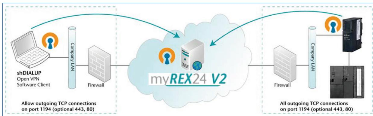
The machine side is connected to the Internet in the same way. Using the WAN interface, the REX router is connected to the customer's router network, establishing a VPN connection to the portal through it. Alternatively, routers are also available that can log in over a mobile connection (3G, LTE).
