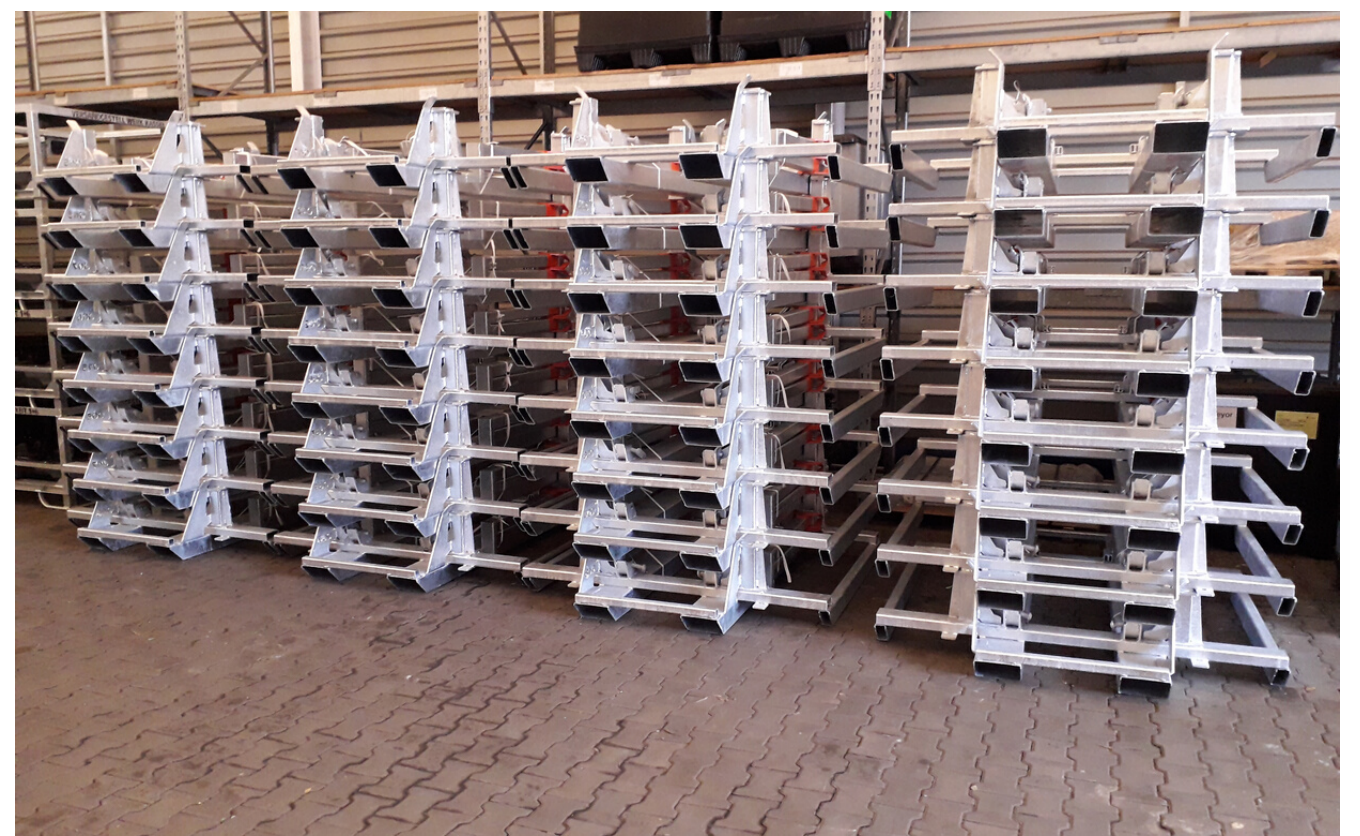
Clip-Lok Steel Racks for transaxles nesting into each other when flat-packed.
