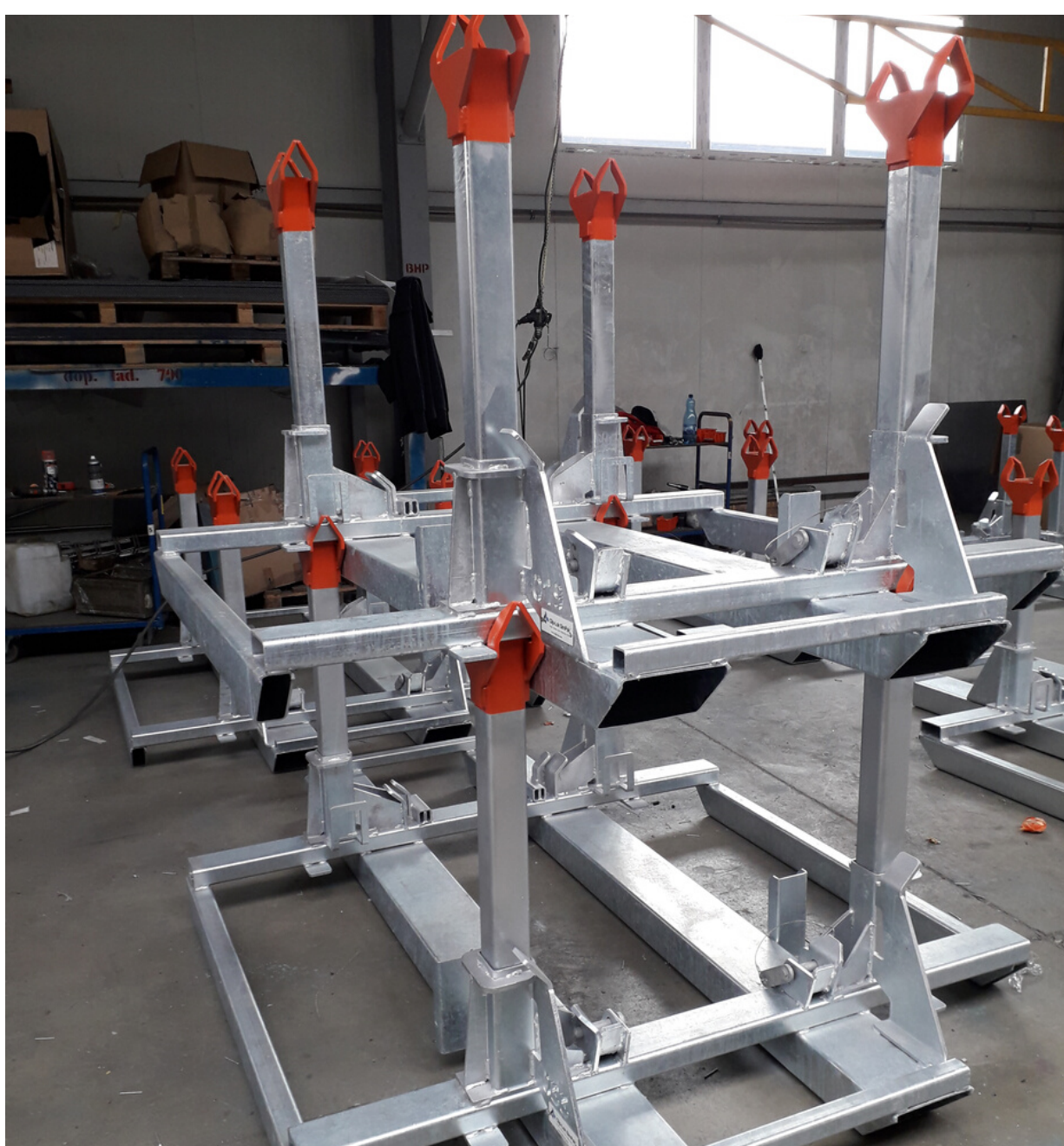
Clip-Lok Steel Racks stacked on top of each other. The top part is coloured orange to make it easy for the operator to see the separation point from the rack to the transaxle.
