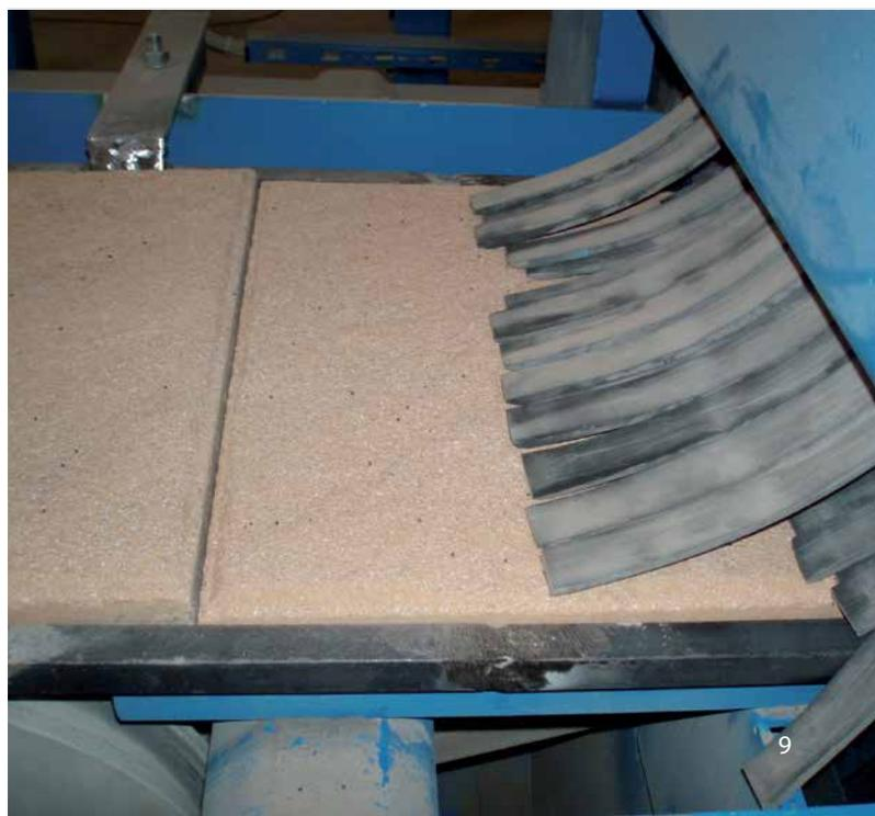
**Wire mesh conveyor shot blast machines** are used for the treatment of a wide range of work pieces. The advantage is that the parts are blasted from both sides at the same time.
