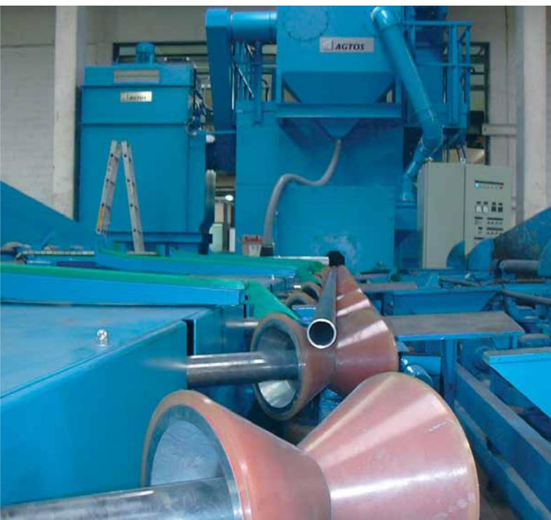
**Diabolo shot blast machines** are used to descale and derust pipes, bars and round sections. As an option, the pipes are freed from the dust and abrasive by means of blowing devices. The special conveyor technology perfectly integrates these machines into the production process. This increases flexibility and ensures a higher output.
