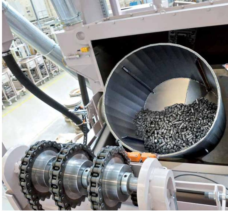
**Travelling grate shot blast machines** are designed for gentle transport of all kinds of work pieces. In this case we show springs being shot peened.
