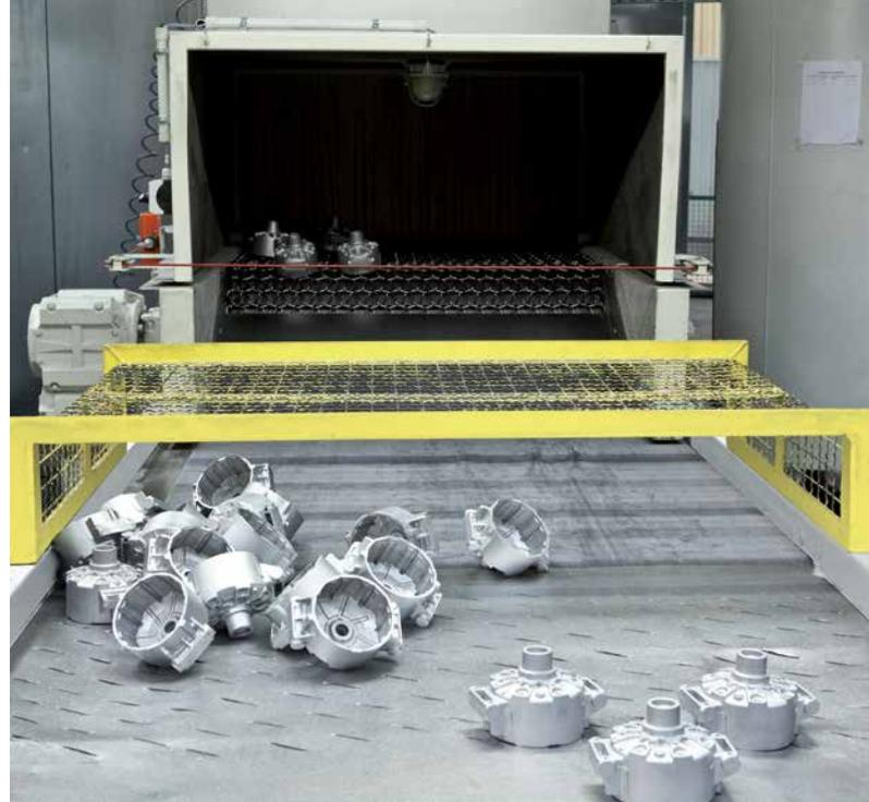
**Walking beam shot blast machines** are used for the treatment of sensitive work pieces. The photo shows quick-release axles prior to blasting.
