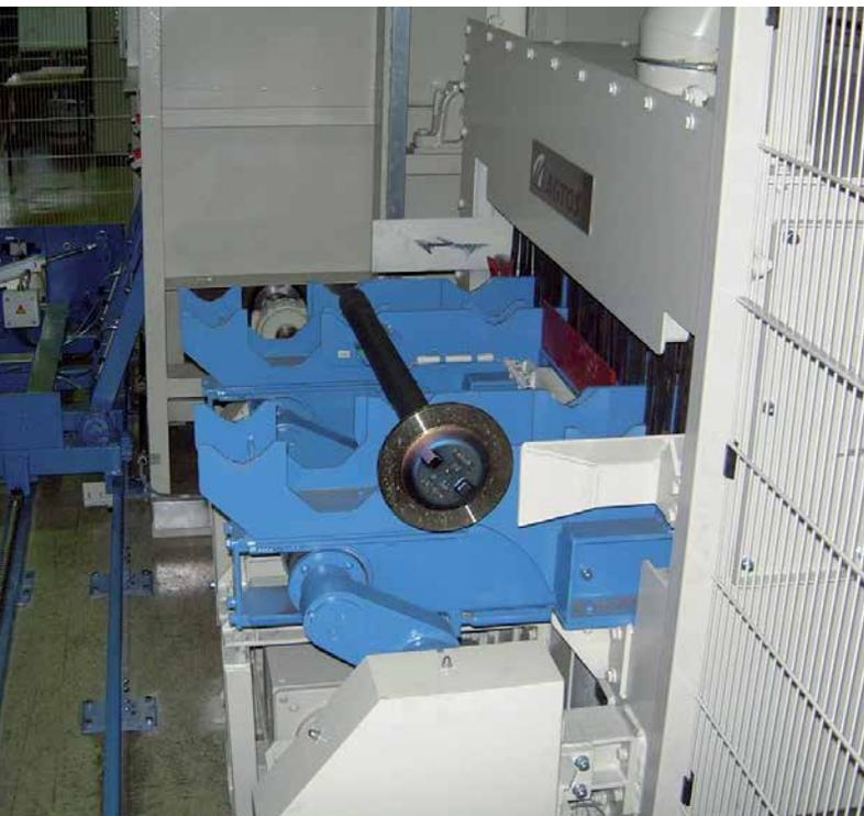
**Overhead rail shot-blast machines** are suitable for a wide range of applications. The work pieces are manually hung up or laid down. The blasting process can be effected in an ideal way by changing the rotational direction and by oscillation of the hangers in front of the turbines.
