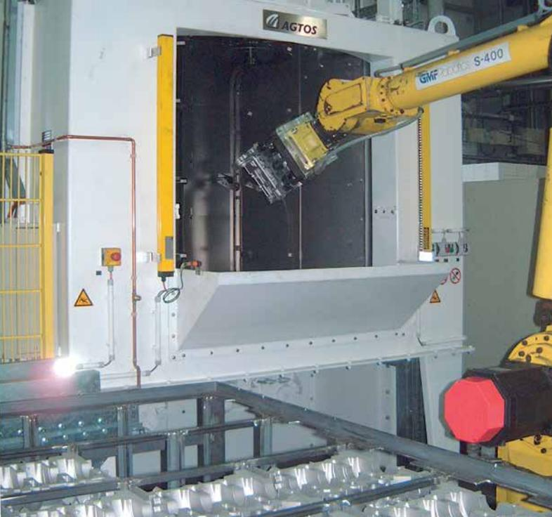
**Rotary table shot blasting machines** are built in different sizes and designs. For shot-peening the automotive industry prefers to use satellite rotary table shot blast machines. Reduced cycle times and reliable blasting results are the result. In addition, they enable automation of the process.
