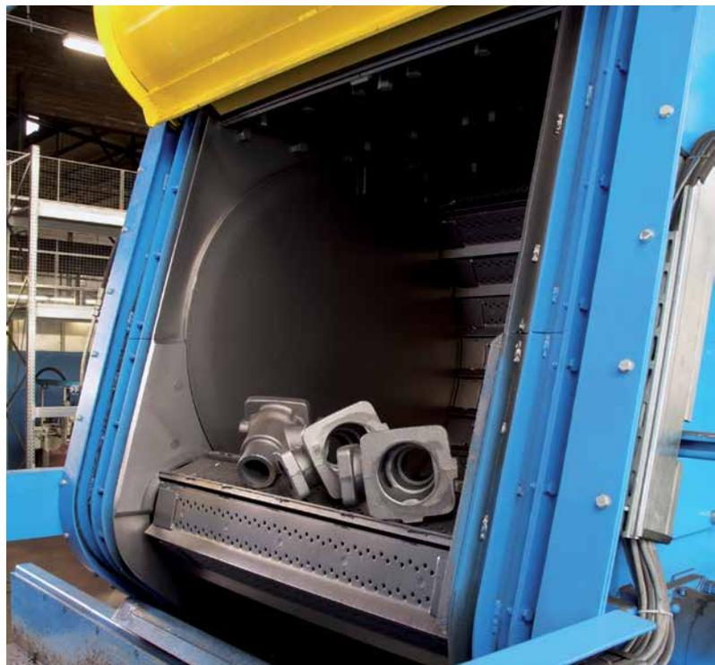
**Roller conveyor shot blast machines** are used to descale and derust profiles, sheets and fabrications. Using cross conveyors, a roller conveyor system can be linked with individual process steps, such as blasting, preservation, sawing and drilling.
