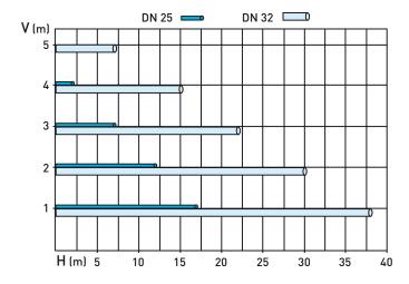
Maximum pipe length allowable for the optimum functioning of the unit. Allowance has been made for two 90° bends and one ABS non-return valve.
