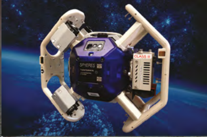
A 3D printed protective bumper for the SPHERES robot operating onboard the International Space Station. Photo source: NASA.
