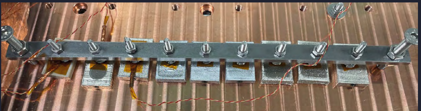
One of the first Z-PEEK samples 3D printed on the Zortrax Endureal successfully covered with metallic coating.
