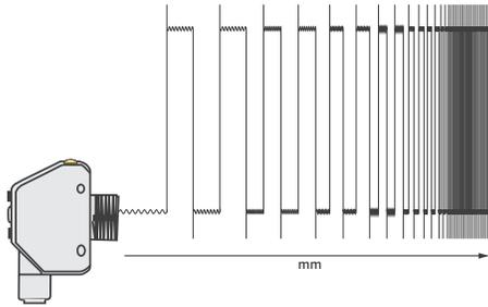
Pulse Pro enables a discrete sensor with PFM output to function like an analog sensor with real time measurement and positioning data
