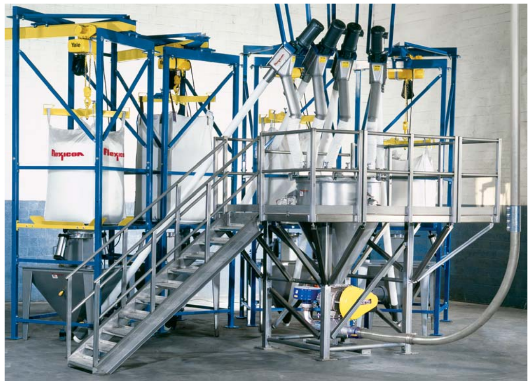
This Automated Weigh Batching System conveys material from Flexicon bulk bag dischargers via Flexicon flexible screw conveyors to a weigh hopper mounted on load cells at mezzanine level. Weighed batches are automatically discharged through a rotary airlock valve into a Flexicon Pneumatic Conveying System, transporting the pre-weighed batch to a blender.
