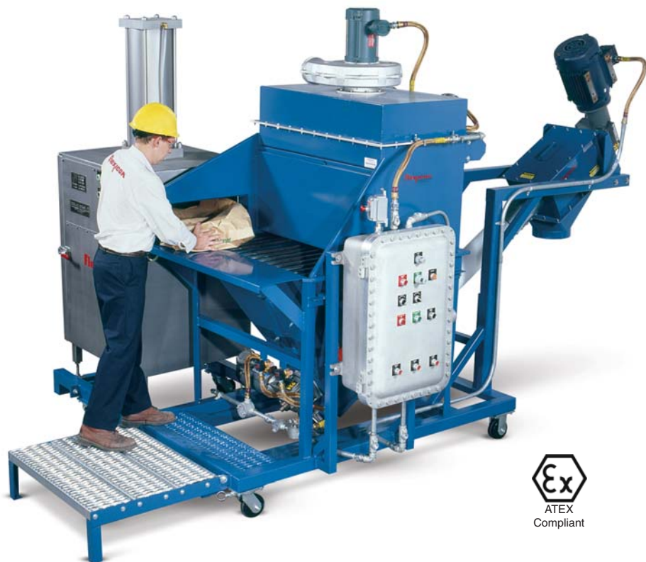
The hoppers of Flexicon Bag Dump Stations are offered with outlets configured for: (left to right) direct connection to process equipment, flexible screw conveyor charging adapters, rotary airlock valves with flow-through adapters, and non-flow-through pick-up adapters for multiple conveying lines.
