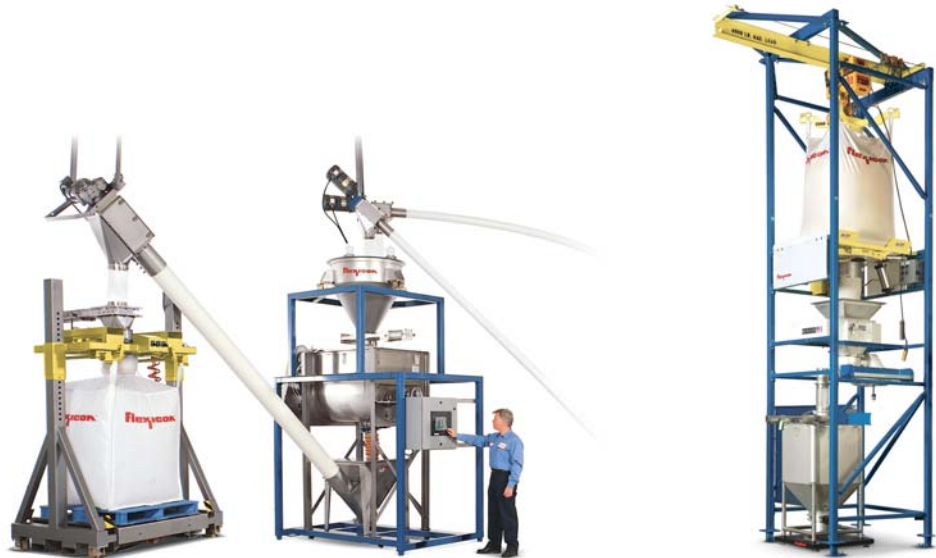
Flexicon's Self-Contained, Gain-in-Weight Batching and Blending System conveys bulk ingredients from multiple upstream sources, weigh-batches, blends and discharges the material into a surge hopper, and transports it to a TWIN-CENTREPOST™ Bulk Bag Filler. The system is offered with Flexicon Flexible Screw Conveyors (shown) or Flexicon Pneumatic Conveying Systems.
