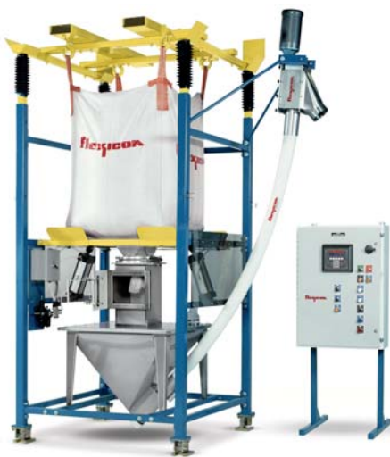
Loss-of-Weight Batching Systems discharge one or more bulk bags while weighing the material and conveying the batch directly to a common hopper, blender, conveyor, shipping container, or any process vessel—automatically and accurately. Load cells transmit the amount of weight lost to a controller, which stops the conveyor once the target batch weight has been reached.
