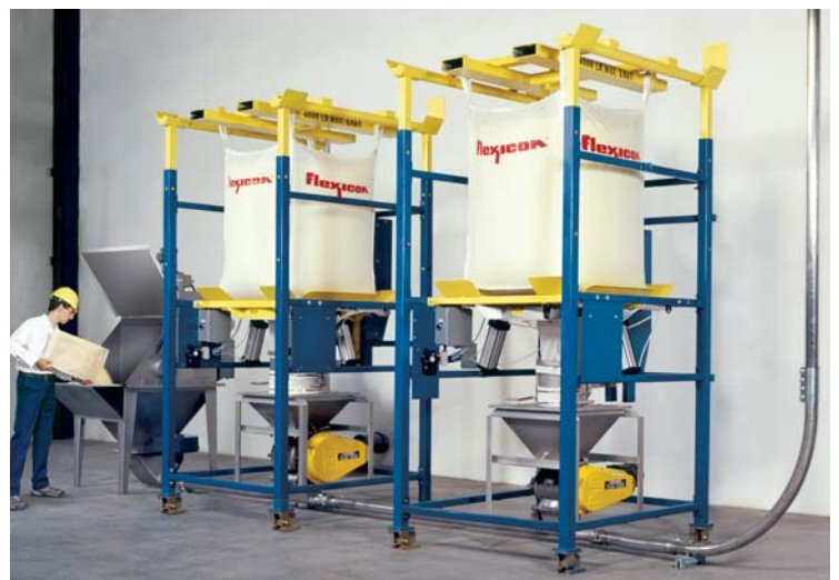
This Loss-of-Weight Batching System conveys material from two Flexicon bulk bag dischargers into a filter receiver which discharges into a blender. The manual bag dump station allows the addition of pre-weighed minor ingredients to the batch.
