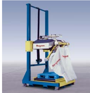
As the entire fill head rises, the bag connection frame is pivoting to a horizontal position.
