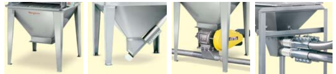
The hoppers of Flexicon Bag Dump Stations are offered with outlets configured for: (left to right) direct connection to process equipment, flexible screw conveyor charging adapters, rotary airlock valves with flow-through adapters, and non-flow-through pick-up adapters for multiple conveying lines.
