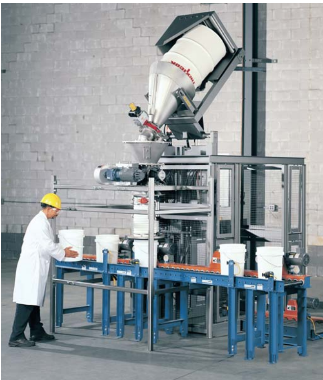
Flexicon's Bulk Filling System with High-Lift Drum Tipper allows drums to be loaded at floor level, sealed against a discharge cone, elevated and tipped, mating the cone spout to a receiver on the filling machine's surge hopper lid. The spout's slide gate valve opens to fill the hopper with no dusting, while pails are indexed, filled by weight, then conveyed to a second scale for check weighing.
