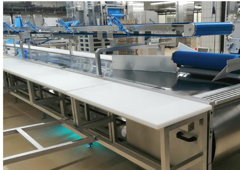
A chrome steel conveyor belt from the Migros meat cutting plant in Gossau with mounted T2018 UVC belt sterilizer
