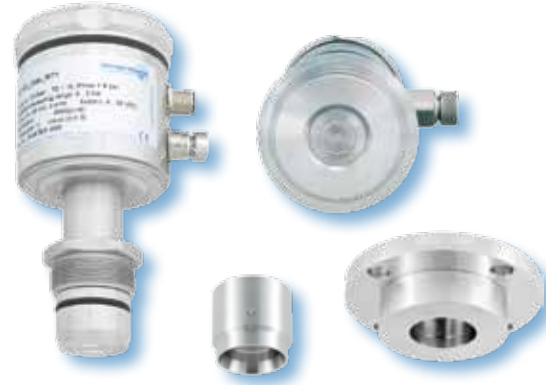
Programmable pressure- and level transmitter PZT 100/101 with flush mounted stainless steel diaphragm, modular connection system, no elastomers
