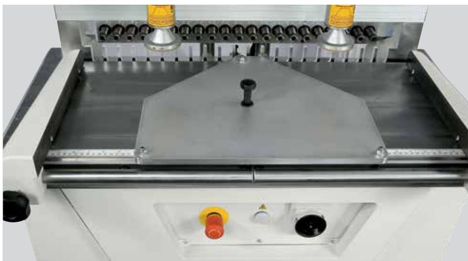
Fence for horizontal boring at  $\pm 45^\circ$ , normally used for  $90^\circ$  joints.
