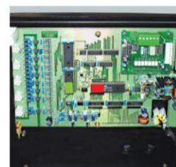
Optional RS485 connection with modbus protocol
