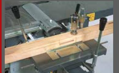
In both directions 2 x 45° mitre cross-cut fence are standard features on the machine.
