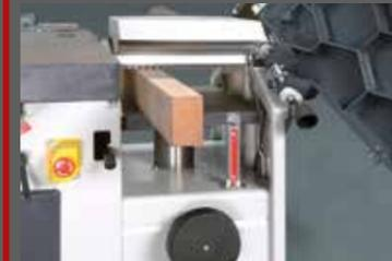
The hard anodized, jointer fence makes edge planing easy. Thanks to its special swivel-support bracket, the fence sets at any angle without a gap between the fence and the table surface.
