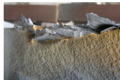
Drawing-step overlap at the end of a bar
