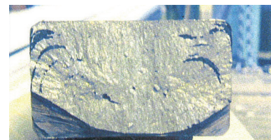
Fracture surface displaying chill
