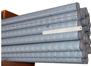
Circumferential drawing marks spaced 55 mm apart
