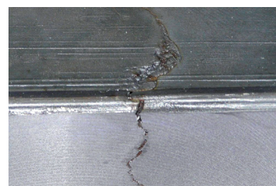
Drawing-step overlap, partially machined
