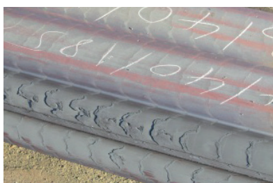
Drawing-step overlaps on a rectangular semi
