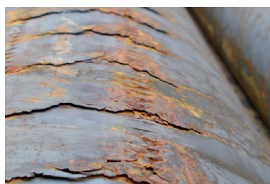
Drawing-step overlap on a round semi
