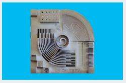
Stereolithography is capable of achieving extremely high detail in parts.
