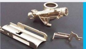
Electroplating has been used for decades to reinforce and structurally stabilize plastic parts. With a high-strength coating, form and fit SL parts can be used as functional prototypes, as well as in low-volume production applications.
