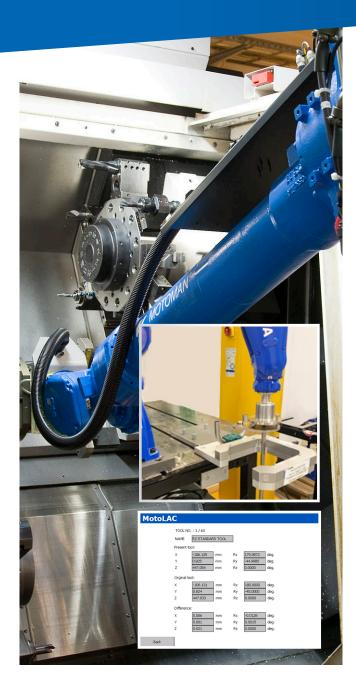
The MotoLAC tool for calibration and automatic correction will ensure a long and trouble-free operation with consistent quality. it will also reduce downtime during a change of tools or after a collision.
