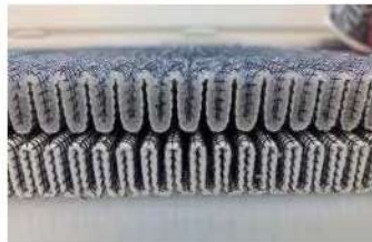
The Filter Media has absorbed water
