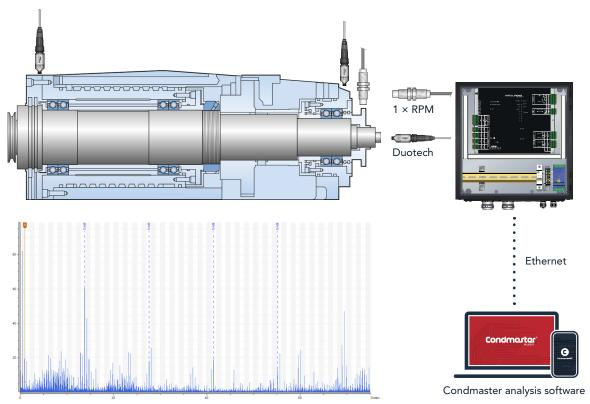
Example of outer ring damage on an 8000 rpm spindle using HD ENV Filter 3.
