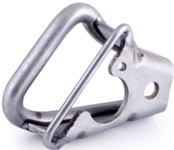
All details are put in a welding fixture and robot welded into a component.
