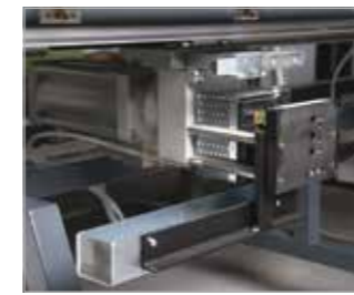
Gear cropper Gear cropper with stops for a centred and consistent handle position. Gear cropper with open cutting tool
