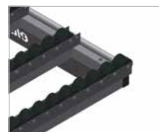
Roller support, compl. for HT 3000/PVC Hard plastic rollers with polyamide coating, on plain bearings, load per roller: 60 kg, convenient for transport and handling of PVC elements HT 3000 Art. no. 250 20 05 33
