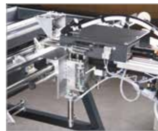
Screwing unit Mobile screwing unit with pneumatic height adjustment. Manual insertion funnel for second screw length. Automatic depth shutoff
