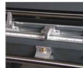
Folding stops (optional) Stop rail with 14 folding stops for constant handle position (7x left, 7x right) FAZ 2800 Art. no. 255 20 63 05
