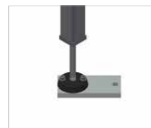
Height adjustment Adjustable height; working height can be set to 850–1,000 mm by means of adjustable feet
