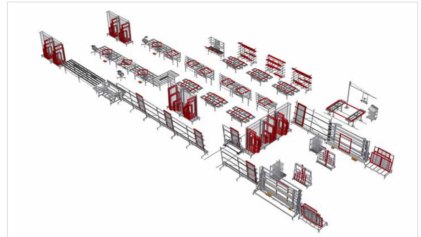
Example of an assembly line for window and door production in aluminium
