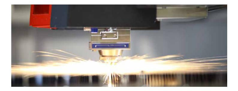
BLS Series Fiber Laser Cutting Machines cover a wide range of industrial applications. Manufactured as "All in One Box" Design structure, the BLS has built in Resonator, Chiller with dual motorized table. A range of fiber power sources starting from 500W to 2500 W are Available. The "BLS" uses new generation high performance linear axis system with high performance rack and high performance class pinion.
